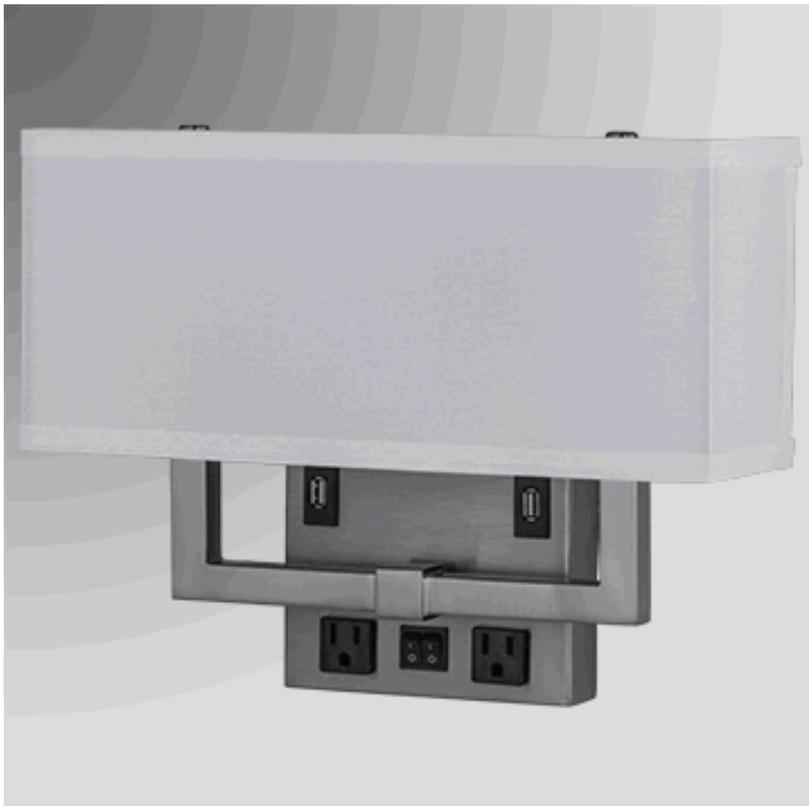
10-5/8"H Brushed Nickel Wall Sconce, two medium base sockets, dual on/off rocker switch at backplate, direct wired, two outlets, two USB ports, 4"x14"x4"x14"x6" White Linen HB Shade. Recommend two 800 lumen LED bulbs.
